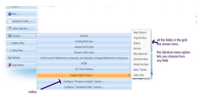
For RVs, in the columns command select "Pretest % CDTP" and you get this critical data point. The "\*\*\*\*" flag for "out of range" is set in the "Configure Pressure Analysis Column". So, you can have it at pretest outside 10% of set pressure, 5%, 3%, etc.
